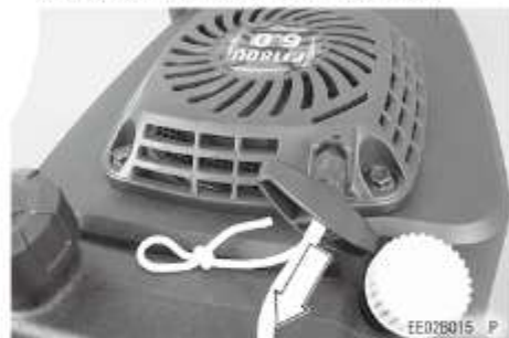
A. Recoil Starter Grip pull in the direction of arrow
