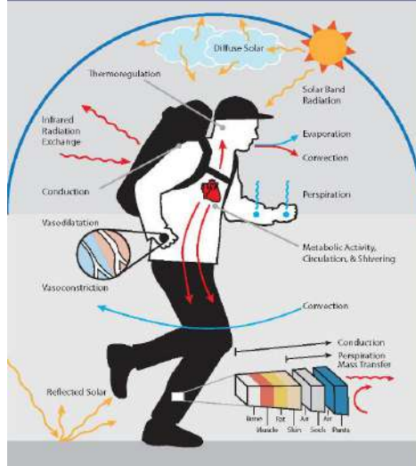
Figure 3. Schematic of ManikinPC 2 Thermoregulatory Control System
