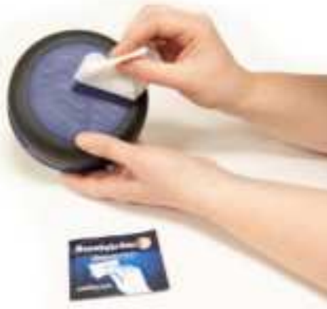
10.4 Clean the pre-filter holders inside and out.
