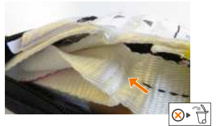
• Absorber has sustained an impact load; absorber has started to tear
