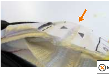
• Absorber has sustained an impact load; absorber has started to tear
