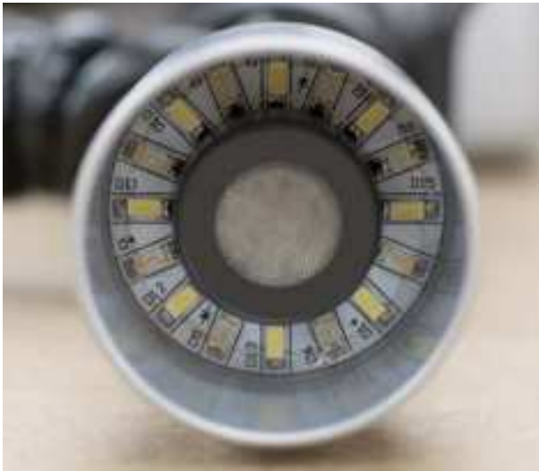
UV and White LEDs arrayed around the Sensor
