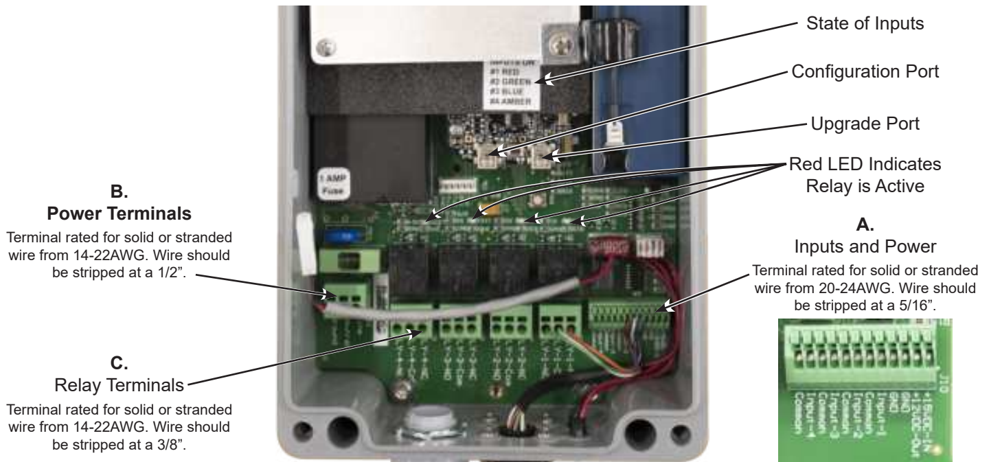
Inside View of MS2000X with -AC, -B, and -LS Options Installed
