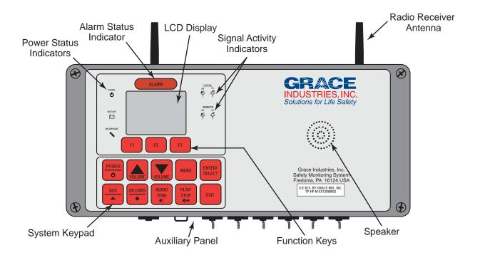
Alarm Status Indicator flashes Red when an Alarm is received.
