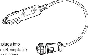
2 Pin connector plugs into 2-Pin Auxiliary Power Receptacle on bottom of SMS Base
