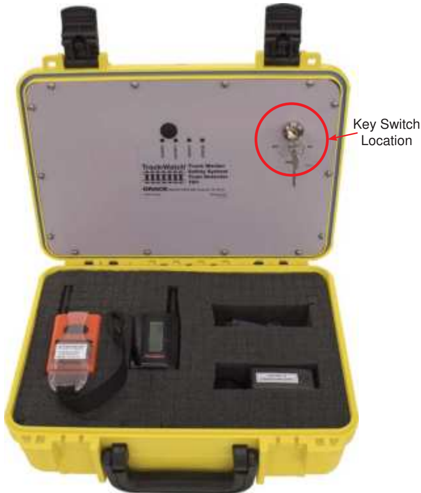
Inside of Train Detector case, shown with Micro TPASS® Repeater and SuperCELL®
