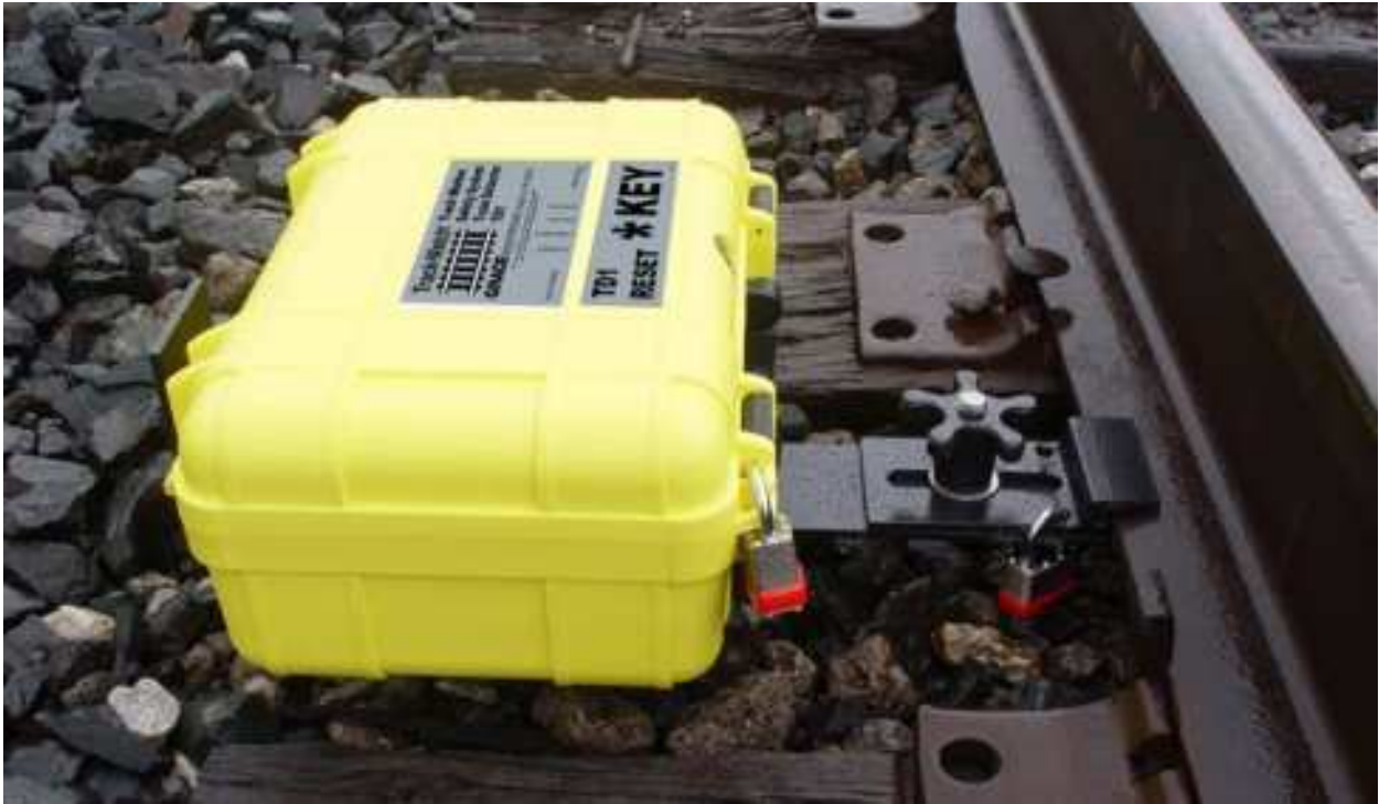
Track-Watch Train Detector mounted to rail
