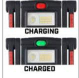
Multi-function push-button switch with battery life indicator
