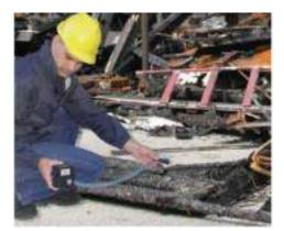
The Model C is a non-calibrated detector used primarily for arson investigation and where it is desirable to detect trace amounts of hydrocarbons.
