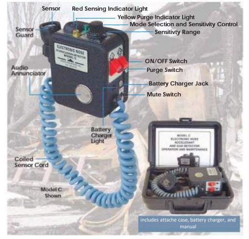
Operation: Turn unit ON, allow several minutes for warm up, and then scan area of concern. When gas or a hydrocarbon is present, beep tones in synchronism with a red indicator light will occur. A slow beep rate indicates a small amount of gas or accelerant, whereas a more rapid rate indicates a higher gas concentration. A mute switch is provided to silence the audio tones and an electronic purge permits rapid recovery of the sensor.
